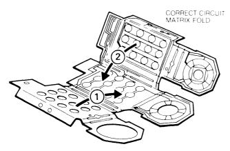
**b)** Install new Circuit Matrix as shown on the front cover.
