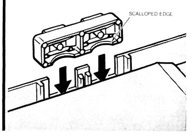
**2** Before you replace the top make sure the Circuit Matrix and the Number Keypad are securely in place so that the top and bottom holes fit over the small brown posts.
