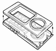
**3** Carefully lift the top off and set it aside. Hold the gold number keypad and the gold direction disc in place with one hand.
